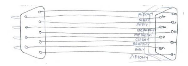
9-pin male and female connectors made by MATT (with contacts in all holes). Wire length 2.0 m
