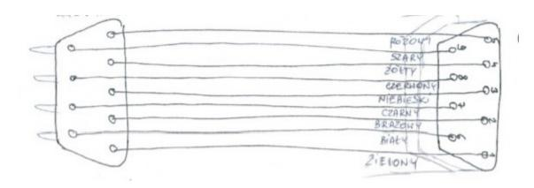
9-pin male and female connectors made by MATT (with contacts in all holes). Wire length 0.1 m
