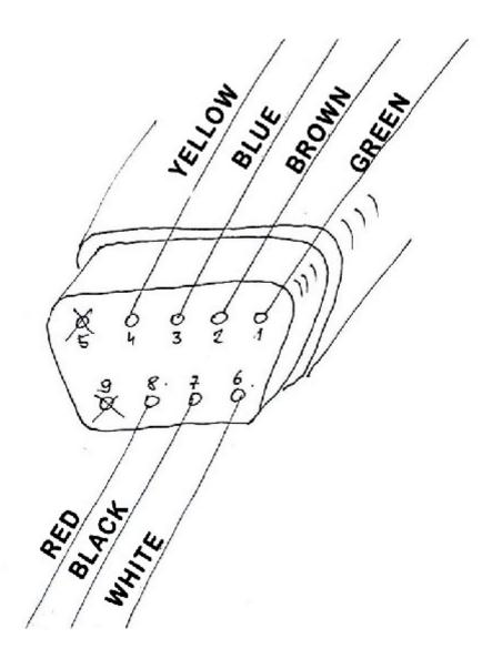
Connecting cable terminated on one side with a 9-pin socket, where 7 pins are used (as shown in the figure above).
