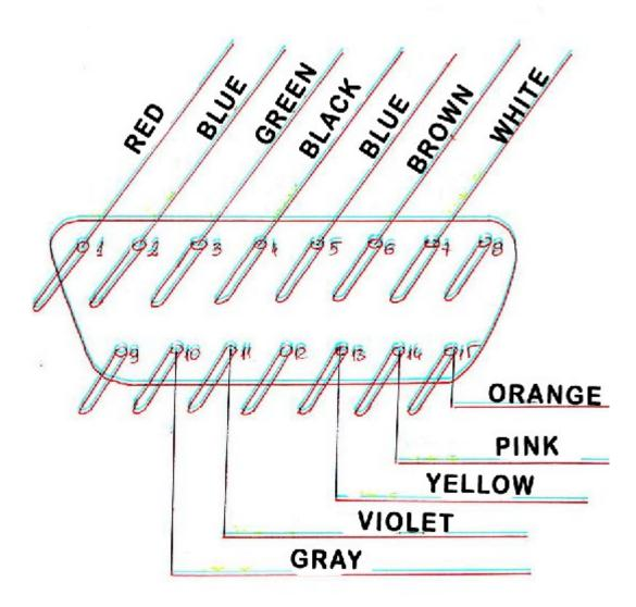
Connecting cable terminated on one side with a 15-pin connector, where 12 pins are used (as shown in the figure above).
