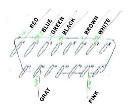
Connecting cable terminated on one side with a 15-pin connector, where 8 pins are used (as shown in the figure above).
