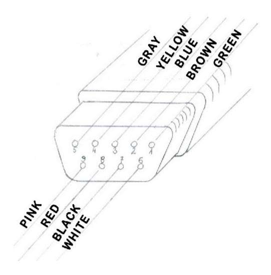
Connecting cable terminated on one side with a 9-pin socket, where 9 pins are used (as shown in the figure above).
