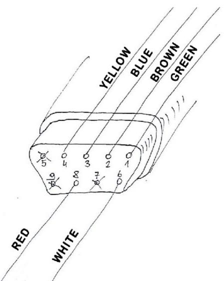
Connecting cable terminated on one side with a 9-pin socket, where 6 pins are used (as shown in the figure above).
