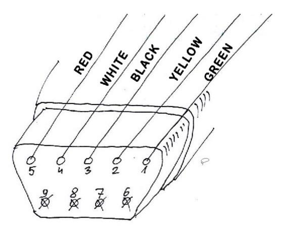
Connecting cable terminated on one side with a 9-pin socket, where 5 pins are used (as shown in the figure above).
