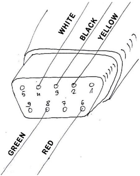
Connecting cable terminated on one side with a 9-pin socket, where 5 pins are used (as shown in the figure above).
