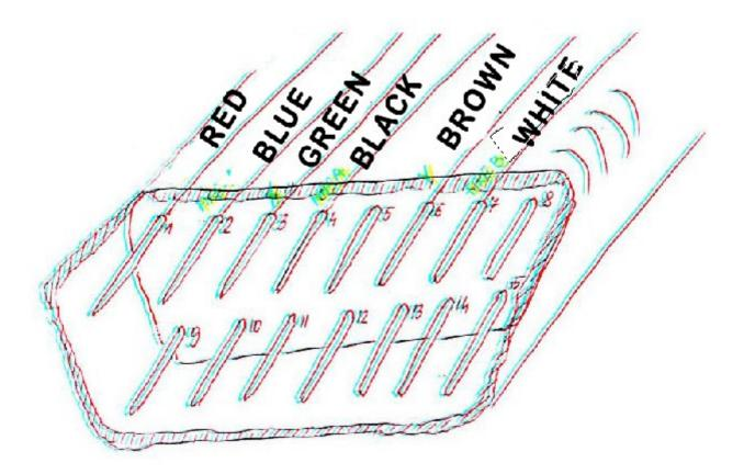
Connecting cable terminated on one side with a 15-pin connector, where 6 pins are used (as shown in the figure above).
