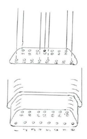
Connecting cable terminated on the one hand with a 15-pin socket, where 7 pins are used (as shown in the figure above).
