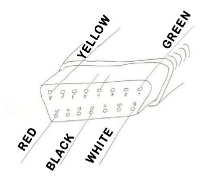
Connecting cable terminated on the one hand with a 15-pin socket, where 5 pins are used (as shown in the figure above).
